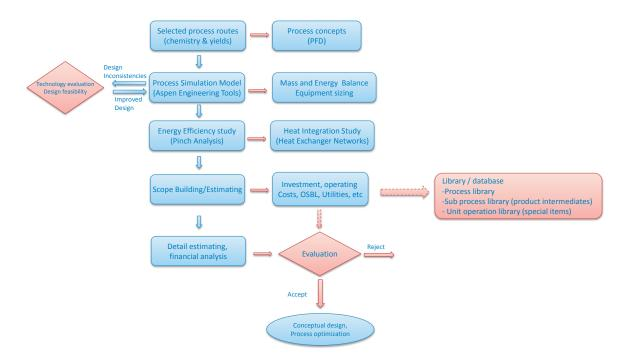
In close cooperation with the company's research experts, Maturus Optimi derives the initial process schemes for each alternative proposed. Using specialized process simulation software tools, fast and reliable technology evaluation is performed for all the process options.
